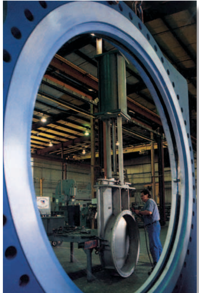
The largest knife gate valve we made in Amory, MS USA had a 96" internal diameter (the area of a 7' x 7' room)
