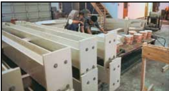
Fabricated Dynaform columns ready for shipment.
