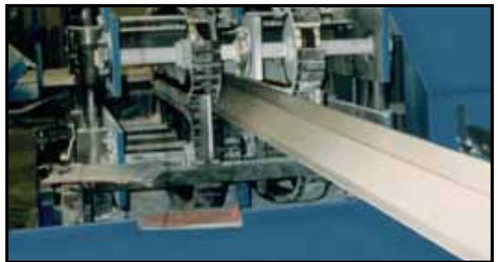
A completed Dynaform shape exits the pultrusion process.
